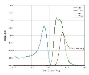
Figure 15: Marginal posteriors obtained for the TPS material, reference material and synthetic silver
