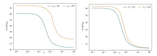
Figure 10: Change on the S-shaped curves positions due to changes in heat flux  $(q_w)$  or wall temperature  $(T_w)$
